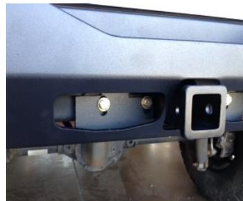
3. Position the R-SE bumper into its desired location using the machined slots on the frame sides. S-SE bumpers are engineered to match the vehicle contour lines; however subtle body difference may occur.
