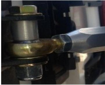
10. Attach the Heim Joint on the swinger side. **\*\* USE 2 1/2" BOLT ON SWING ARM SIDE)**
