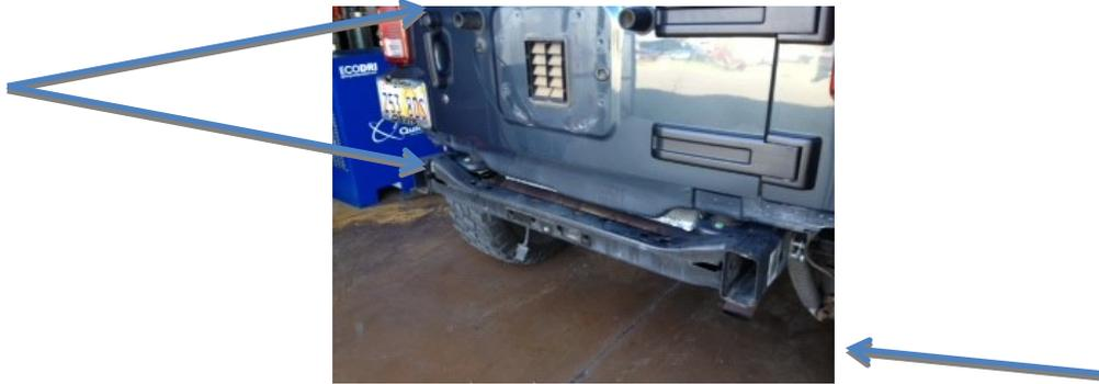
Arrows indicate frame side bolts (2 per side) and tire carrier (4 per side)
