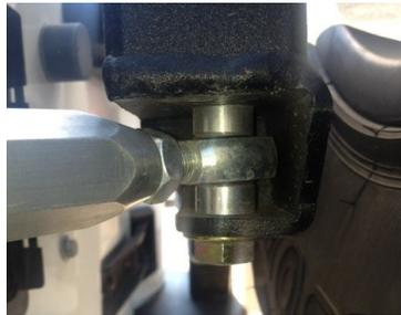
11. Combine the tailgate and swinger sides using the turnbuckle.
